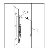
Use the Locking bar(4) to prevent the TV from being removed or accidentally knocked off of the wall plate. When the locking bar half insertes into the wall plate, you can use the rotating rod(5) to make it fully inserted.
